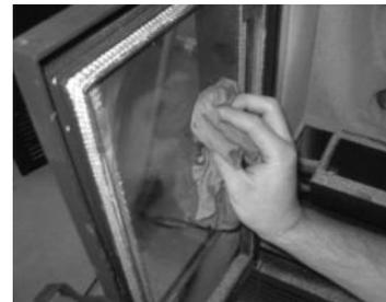
Figure 10 – Cleaning of the glass: a) moisten a soft cloth with liquid; b) clean the glass with the cloth
